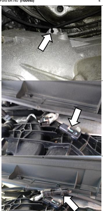
Install supplied zip-ties to support the wiring harness.
