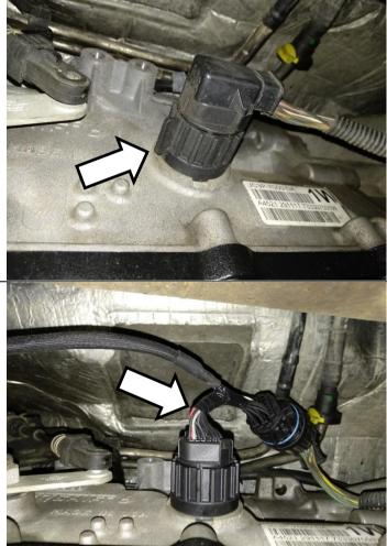
Route the supplied BD harness to the transmission and connect it inline.
