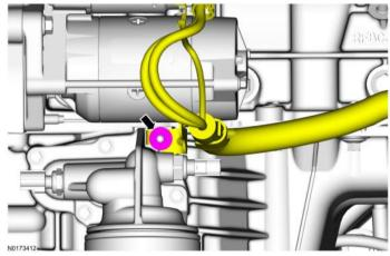
12. If equipped, disconnect the block heater cord.
