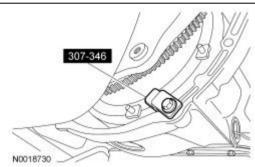
Position the transmission on the dowel pins on the back of the engine. Install the 11 bolts. Tighten to 48 Nm (35 ft-lb).
