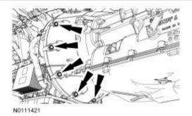
37. Slide the transmission back enough to install the Torque Converter Retainer and remove the transmission.
