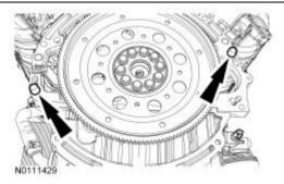
2. Lubricate the torque converter pilot hub with multi-purpose grease and align the paint dot on the torque converter in the 12 o'clock position.
