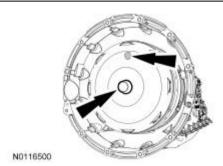
3. Install the Torque Converter
