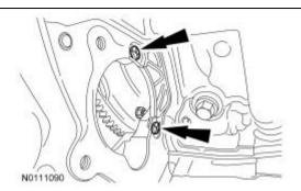
7. Install a new transmission fluid filler tube O-ring. Lubricate it with clean transmission fluid.
