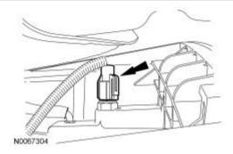
28. For vehicle with electric shift transfer case; disconnect the gearmotor encoder connector and the gearmotor electrical connector.
